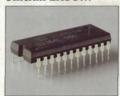
The new 8K BASIC ROM used in the Sinclair ZX81 is available to ZX80 owners as a drop-in replacement chip. (Complete with new keyboard template and operating manual.)
